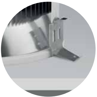
Mounting ring made of steel with fitting spring for ceiling installation without tools for ceiling thicknesses of 1–30 mm Bayonet connection for reflector
